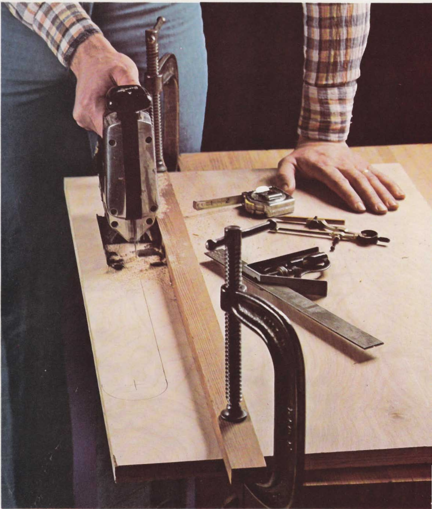
Careful marking and cutting along a guide ensure precise work. Versatile saber saw is one of the most useful cutting tools.
