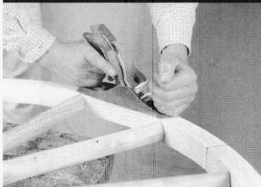
The face side of the felloes is planed, so that all their faces lie flat and true with one another.
