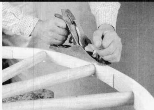
A smoothing plane is used to clean up the cut made by the power plane.
