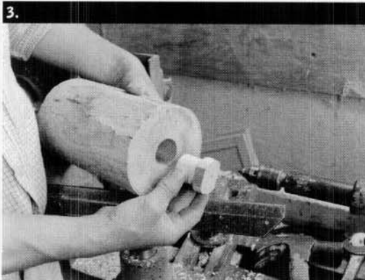
The chopped stock is mounted on the lathe, here a turned plug is inserted to the pilot hole.
