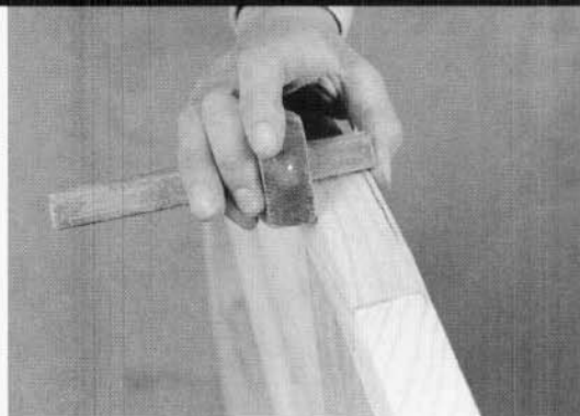
The sole is marked with a marking gauge.
