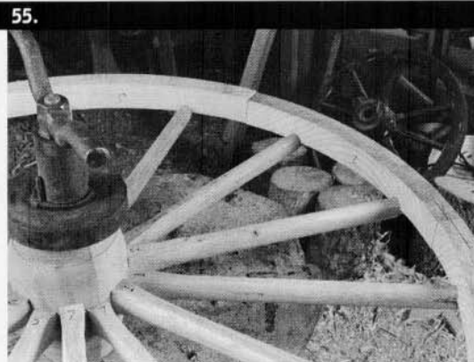
55. Here the felloes are numbered, note the line across the felloe-joint.
