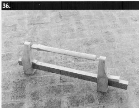
36. The spoke fiddle. The spoke is secured between the points. The spoke is marked out with a centre line down the face side, and lines on the edges of the face.
