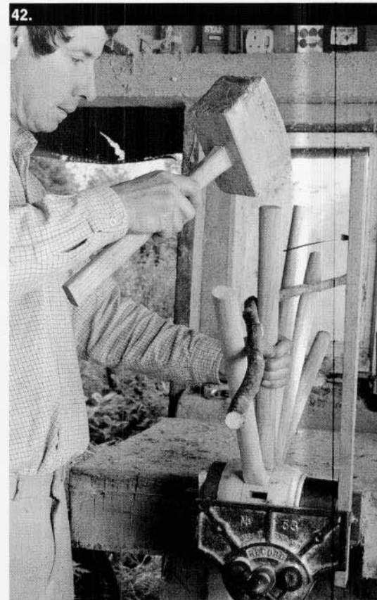
42. The spoke bridle in use, here it is pulling the spoke which is being driven forward.
